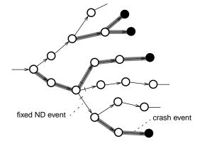
**Figure 7:** Portion of a state machine, its crash events, and corresponding dangerous paths. Crash events are those that end in states filled black. Fixed non-deterministic events are marked with a slash. The shaded paths are dangerous.
