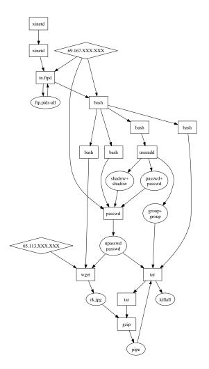
Figure 2: Tracking the FTP intrusion.
