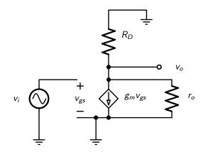
$$v_o = -g_m v_{gs}(R_D||r_o)$$
