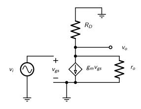
$$v_o = -g_m v_{gs}(R_D||r_o)$$
