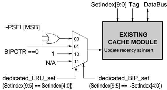
Figure 16: Hardware changes for implementing DIP
