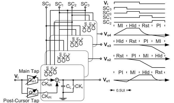
Fig. 3. The overall AAF/FFE system block diagram.
