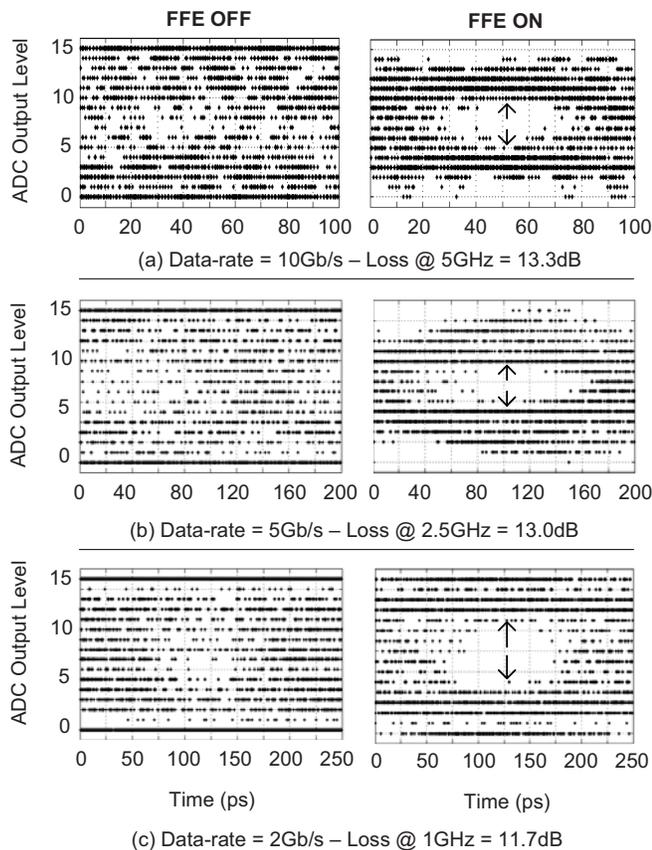
Fig. 9. Digital eye-diagrams with FFE OFF/ON.
