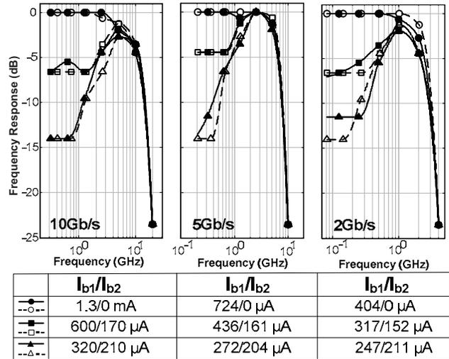
Fig. 7. Measured (solid) vs simulated (dashed) frequency response.
