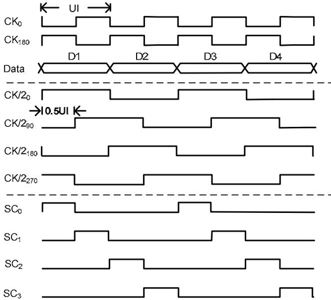
Fig. 6. Clock timing diagram.
