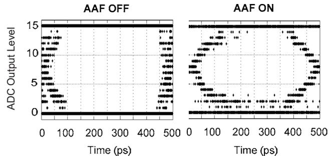
Fig. 8. Digital eye-diagrams with AAF OFF/ON.
