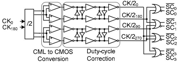
Fig. 5. The clock generation circuitry.
