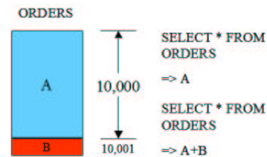
Figure 4. Incremental change for a query response (A) upon inserting a new row (B)
