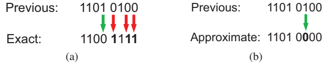
Fig. 3: Example of using FLIPBIT to perform an approximate store. (a) For the exact write, we require expensive 0 to 1 transitions (red arrows). (b) For the approximate write, we only use inexpensive 1 to 0 writes (green arrows).
