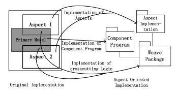
Fig. 1. Code transformation for the aspect-oriented refactorization.
