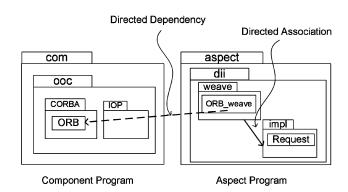
Fig. 2. Package organization for aspect-oriented refactorization.
