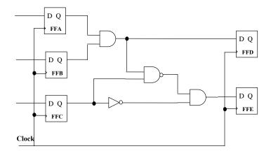
(a) [4] Determine the minimum clock period for which this circuit is guaranteed to operate correctly. Show how you arrived at your answer.
