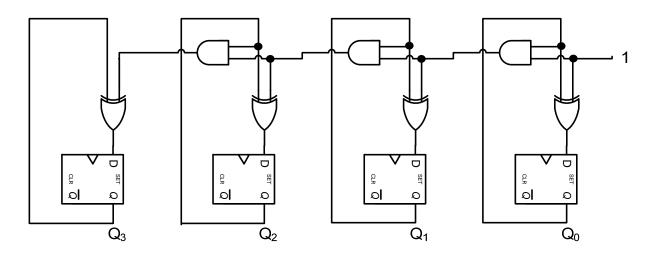
[3] (i) Determine the minimum amount of time that it takes for this counter to count from 0 (i.e.  $Q_3Q_2Q_1Q_0 = 0000$ ) to 15 (i.e.  $Q_3Q_2Q_1Q_0 = 1111$ ).
