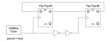
[2] (iii) Assume that each inverter has a delay of 0.5 ns. If this circuit is still to work correctly, what is the largest value that the hold time for the flip-flop labeled Flip Flop #2 can be?
