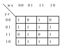
You are to derive a number of covers for f from the above K map, but not necessarily of the lowest cost. All covers are required to be either sum-of-products or product-of-sums. The cost is calculated as (the number of gates) + (the number of inputs to gates). Inversion of an input variable has no cost.
