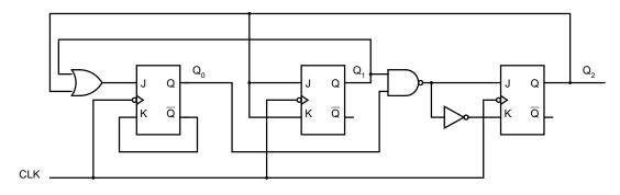
Draw a timing diagram (four complete clock cycles) for  $Q_0$ ,  $Q_1$  and  $Q_2$ . Assume that all initial values are 0. Note that all flip-flops are negative edge-triggered.
