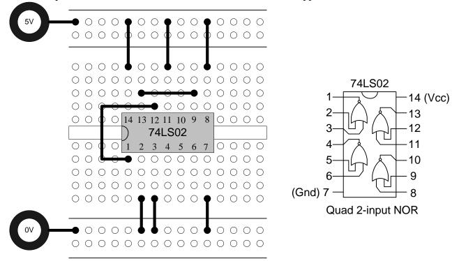
(a) Draw the schematic of the digital circuit that is wired, using the value "1" to represent logic 1 and "0" to represent logic 0 where ever it appears.
