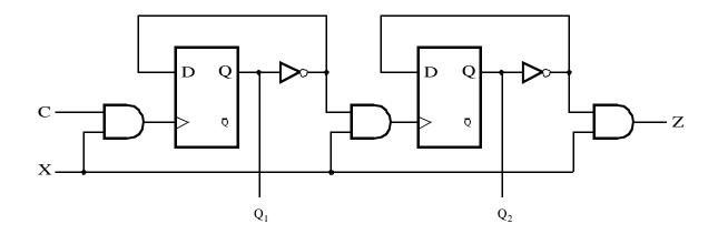
(a) [4] Assuming zero delay time through both logic gates and flip-flops, complete the timing diagram shown below. Note that we assume both flip-flop outputs are 0 to start.
