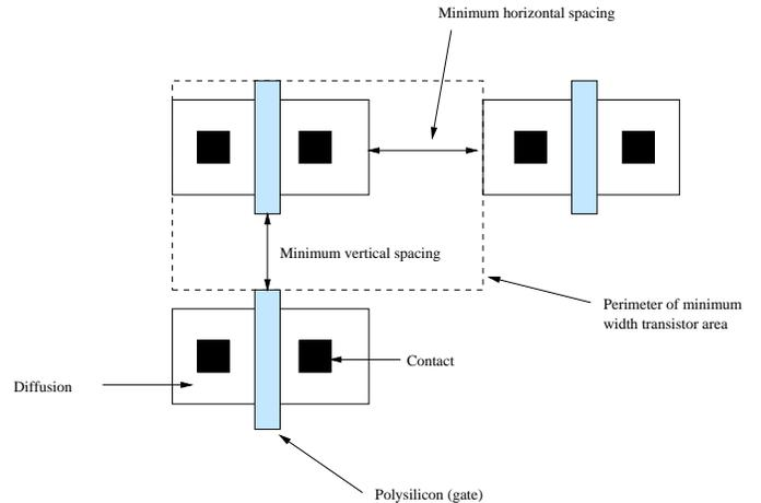
Figure 4: Definition of a Minimum-Width Transistor Area [4]
