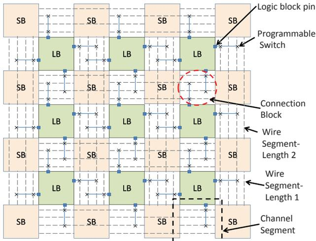
**Fig. 1.** FPGA Architecture and Related Terminology.
