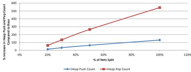
**Fig. 10.** Increase in Heap Push and Pop Count as a function of amount of pin-to-wire routing
