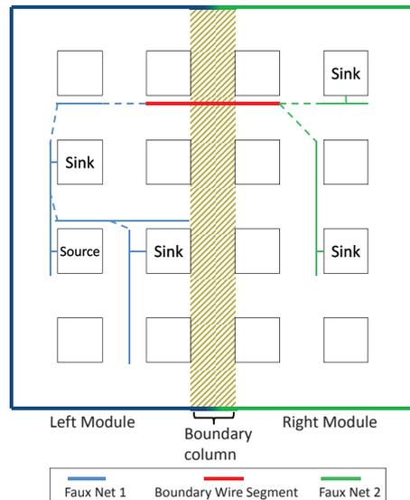
**Fig. 4.** Faux-Nets built from Net shown in Figure 3 now with just one crossing point
