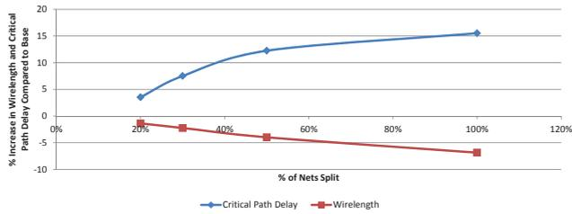
**Fig. 9.** Percentage variation in total wirelength and critical path delay as a function of amount of pin-to-wire routing
