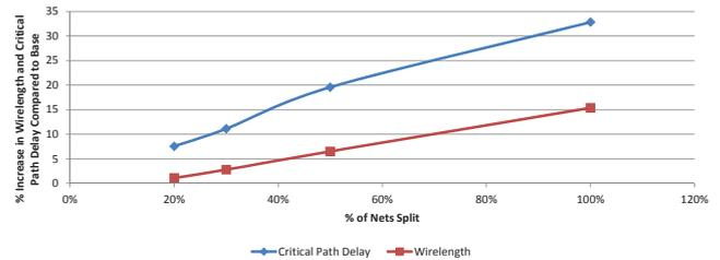
**Fig. 11.** Percentage variation in total wirelength and critical path delay as a function of amount of pin-to-wire routing - Harder Dispersed Routing
