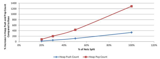
**Fig. 12.** Increase in Heap Push and Pop Count as a function of amount of pin-to-wire routing - Harder Dispersed Routing
