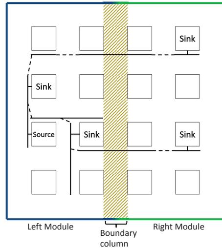
**Fig. 3.** A Multiple Crossing Double-Sided Net in the Original Netlist
