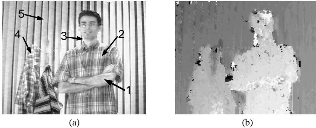
Figure 4.12: (a) Input from right camera, (b) Output disparity map
