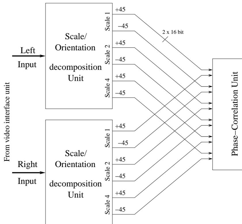
Figure 3.8: Communication between Scale/Orientation Unit and Correlation Unit
