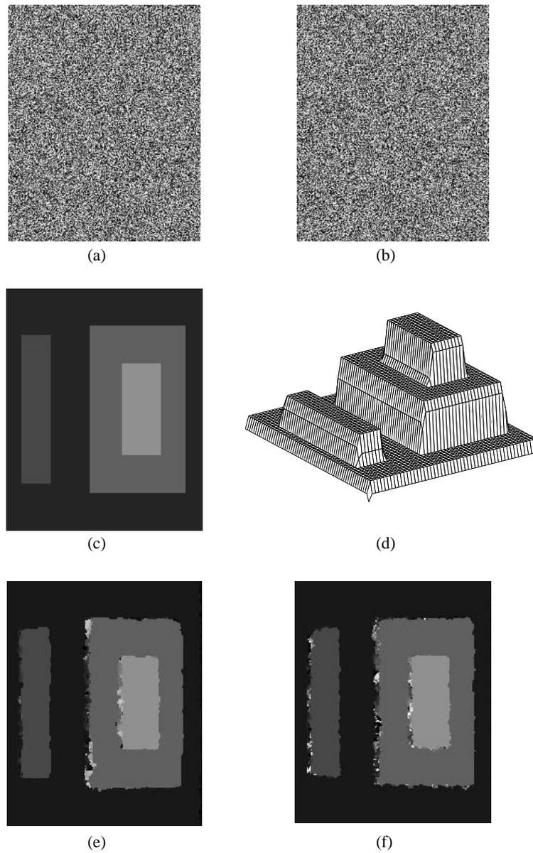
Figure 4.11: Overall system performance on a pair of random stereograms: (a), (b) Random-dot stereogram (c) Ground truth depth (d) 3D structure of ground truth (e) Depth from original software (f) Depth from hardware vision system
