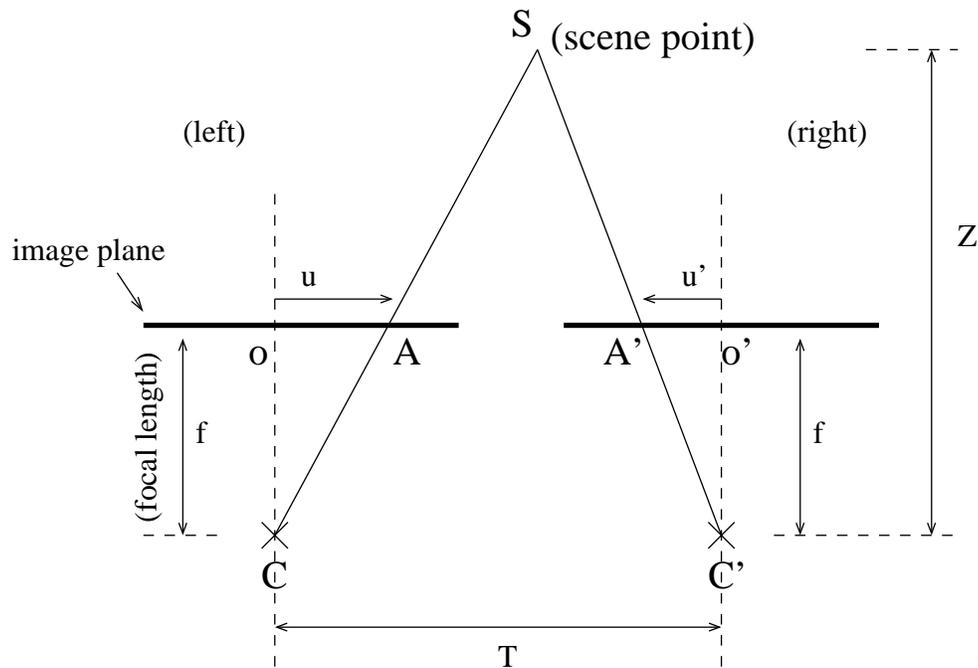
Figure 2.2: Calculating depth from disparity
