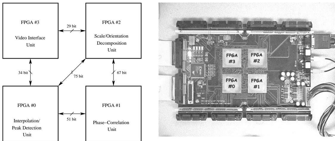
Figure 3.23: Data transfer between four FPGAs
