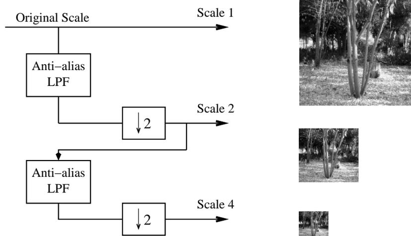
Figure 3.4: Two-step scaler architecture with anti-alias low-pass filters and 2D down sampling
