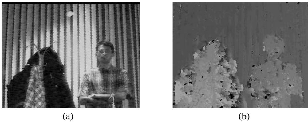
Figure 4.16 (a) Input from right camera, (b) Output disparity map
