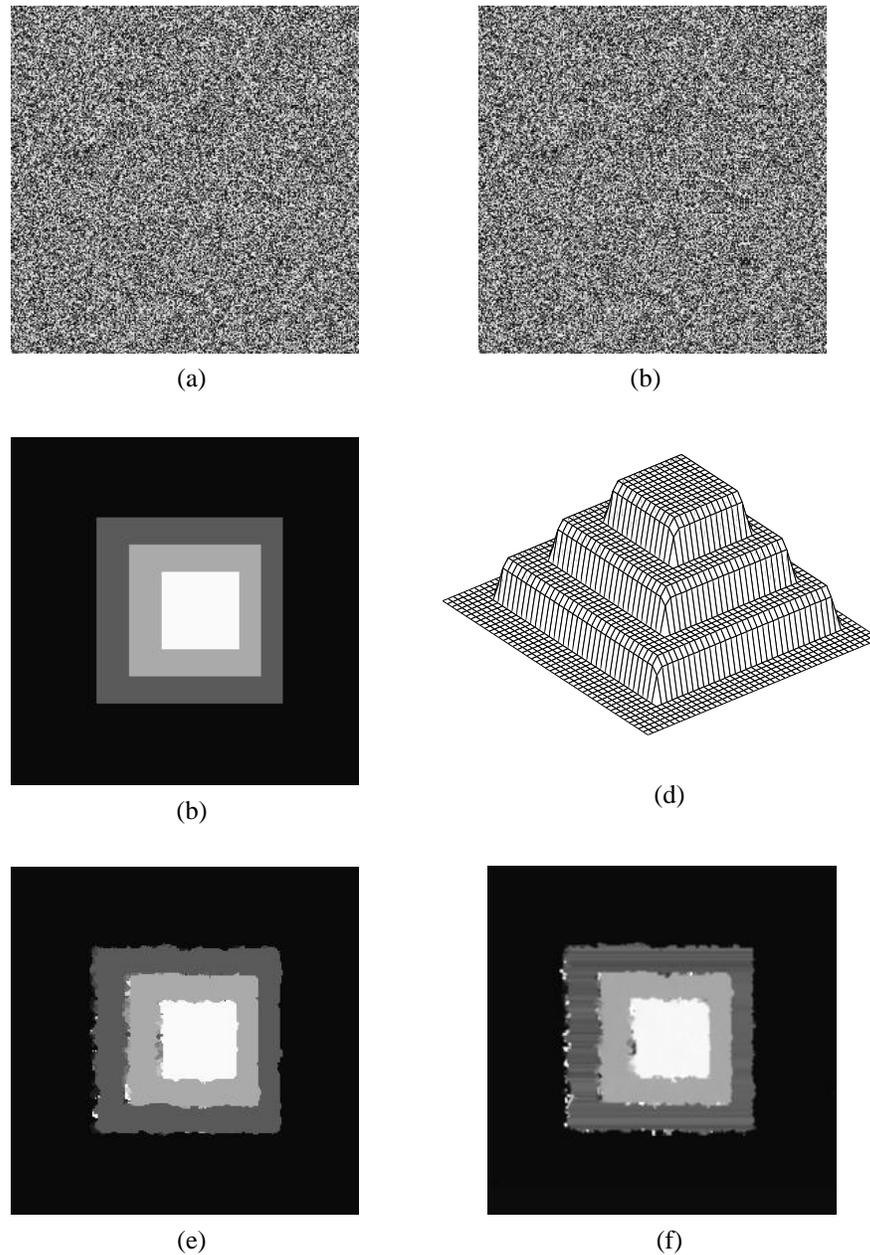
Figure 4.10: Overall system performance on Wedding-cake random stereograms: (a), (b) The stereogram (c) Ground truth depth (d) 3D structure of ground truth (e) depth from original software (f) depth from hardware vision system
