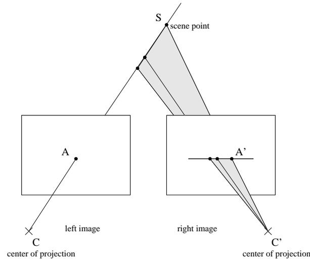
Figure 2.3: Epipolar Constraint
