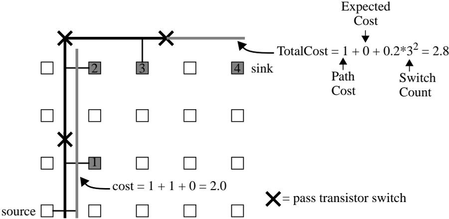
**Figure 3.13:** Example of SwitchCount
