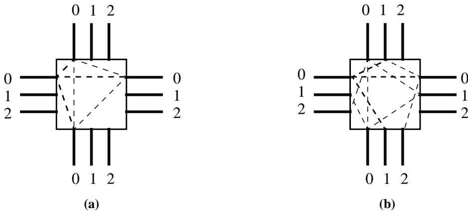
**Figure 2.2:** Switch boxes: (a) planar, (b) non-planar Wilton [5]
