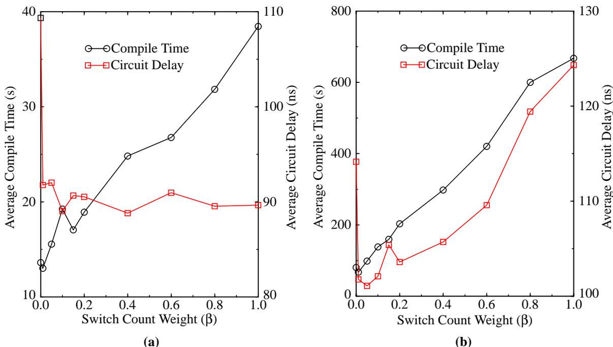
**Figure 3.14:** Average compile time vs.  $\beta$ , (a) low-stress routing problems, (b) difficult routing problems, for 4000X-like architecture
