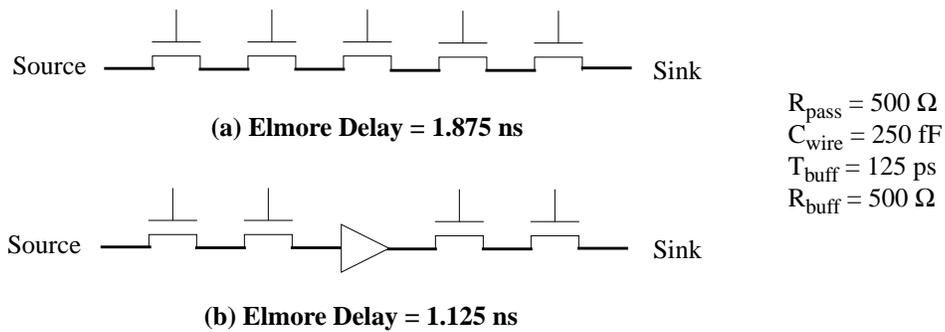
**Figure 3.11:** Examples of routing use pass transistor and buffered switches
