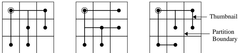
**Figure 2.6:** Three possible thumbnails for a  $3 \times 3$  partitioning [20]
