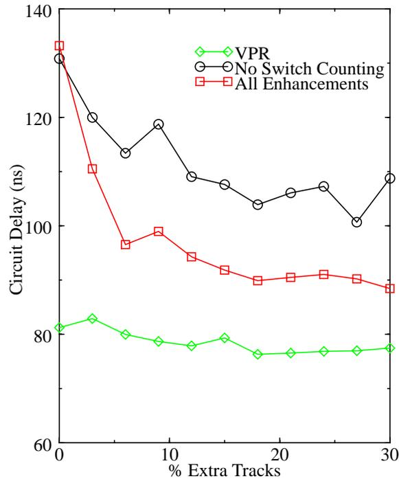
**Figure 4.3:** Circuit delay vs. % extra tracks
