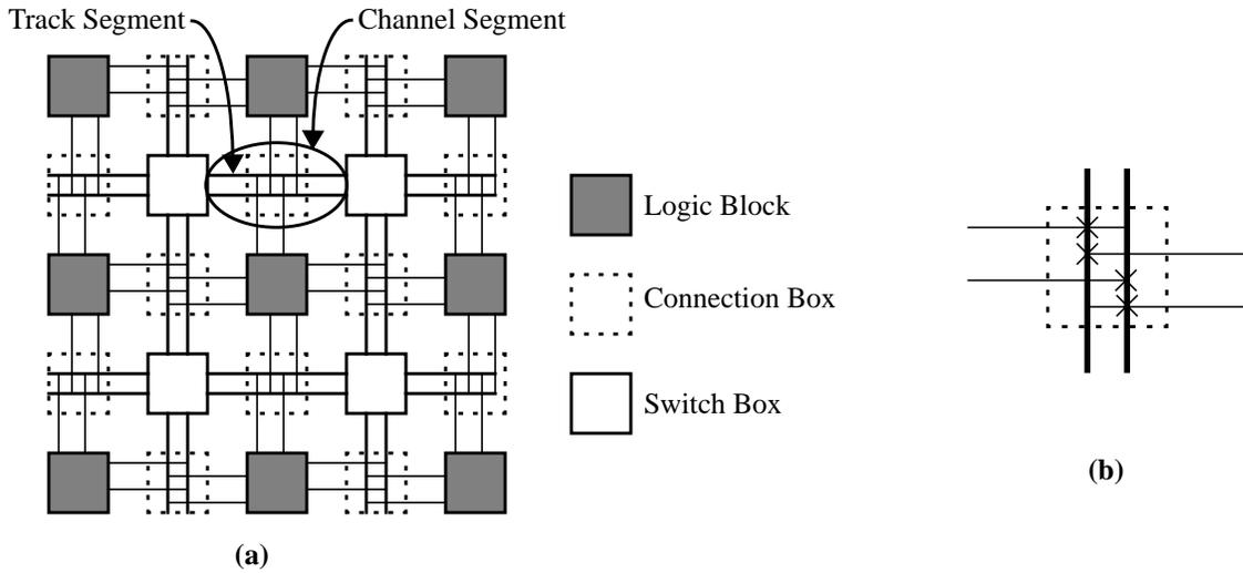
**Figure 2.1:** (a) Island-style FPGA architecture, (b) connection box
