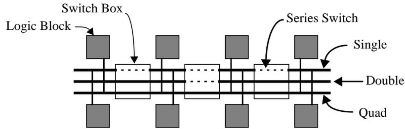
**Figure 2.3:** Example of segmented routing architecture
