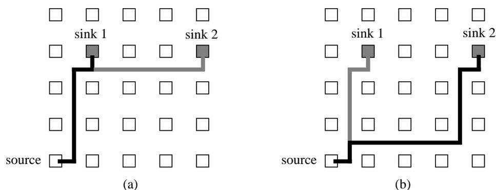
**Figure 3.7:** Two methods of routing a multi-terminal net: (a) closest sinks first, (b) furthest sinks first
