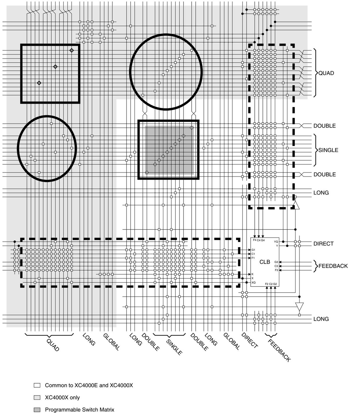
**Figure 2.10:** Detailed view of routing for a logic block [28]
