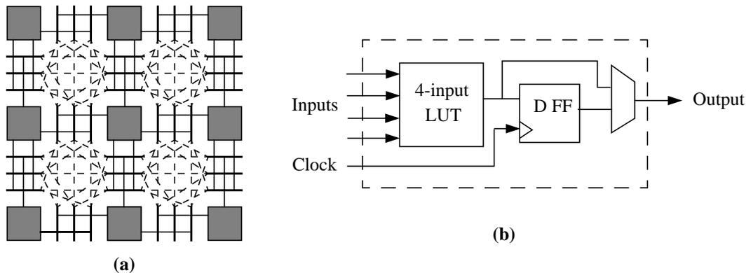
**Figure 3.1:** (a) Simple FPGA routing architecture, (b) Simple FPGA logic block
