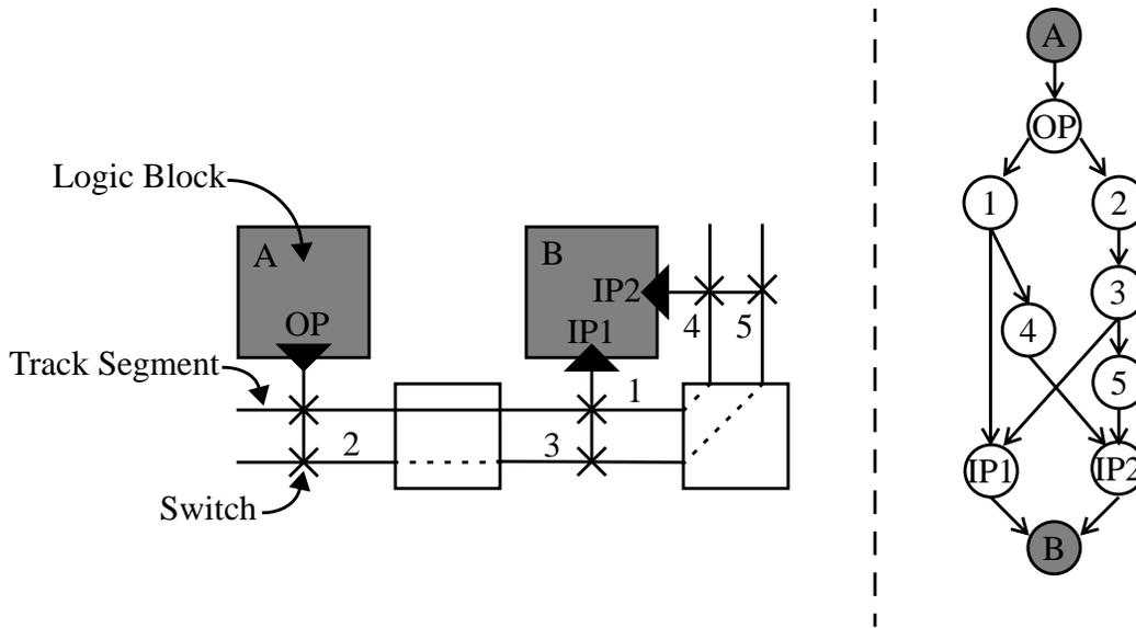
**Figure 2.4:** FPGA routing architecture and graph representation
