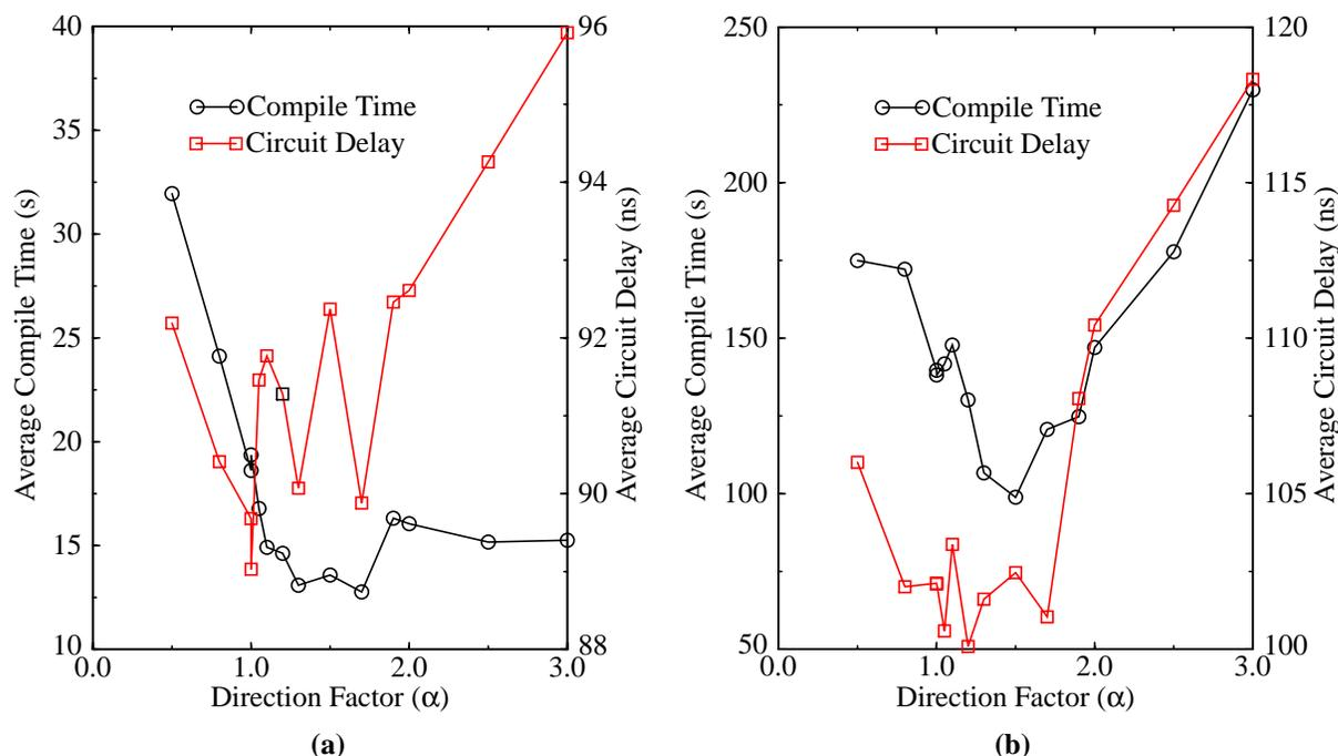
**Figure 3.6:** Compile time and circuit delay vs.  $\alpha$ , (a) low-stress routing problems, (b) difficult routing problems, using the 4000X-like architecture
