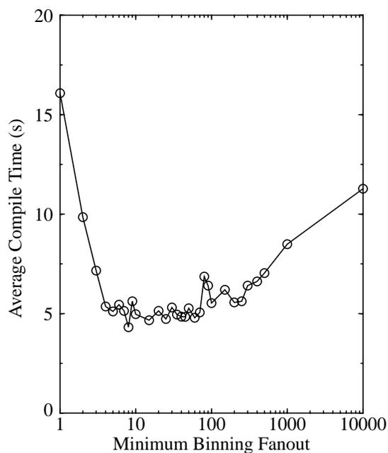
**Figure 3.9:** Average low-stress compile time vs. minimum binning fanout
