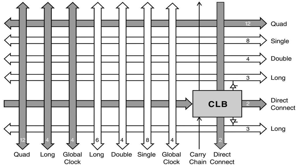
**Figure 2.9:** Overview of routing for a logic block (shaded = 4000XL only) [28]
