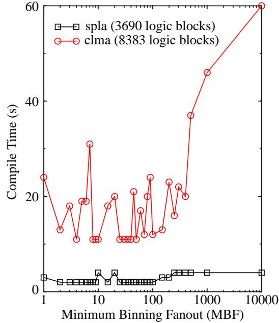
**Figure 3.10:** Low-stress compile time vs. minimum binning fanout for circuits *spla* and *clma*
