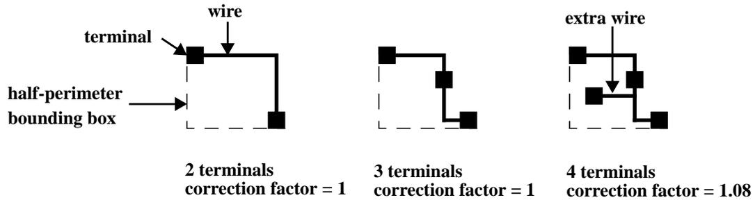
**Figure 2.7:** Examples of correction factors
