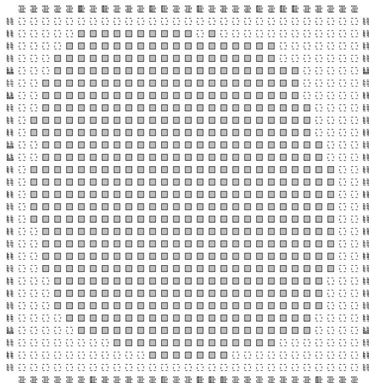
**Figure 5.1:** Placement from VPR with 30% extra logic blocks
