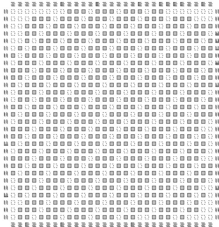
**Figure 5.3:** Placement with 30% extra logic blocks placed in diagonals
