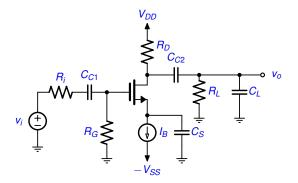
Capacitors C<sub>C1</sub>, C<sub>C2</sub>, C<sub>S</sub> are low freq caps and are all shorted for high frequency analysis
