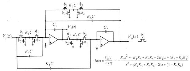
Given  $C_1 = 1\,\mathrm{pF}$  and  $C_2 = 3\,\mathrm{pF}$ , find the values (in pF) for  $K_1C$  to  $K_6C$  so that  $H(z) = -\frac{0.288(z-1)}{z^2-1.572z+0.9429}.$  Note that the subscript "j" on  $K_iC_j$  has been deleted on the above figure so that you need to determine which integrating cap to reference the value to.
