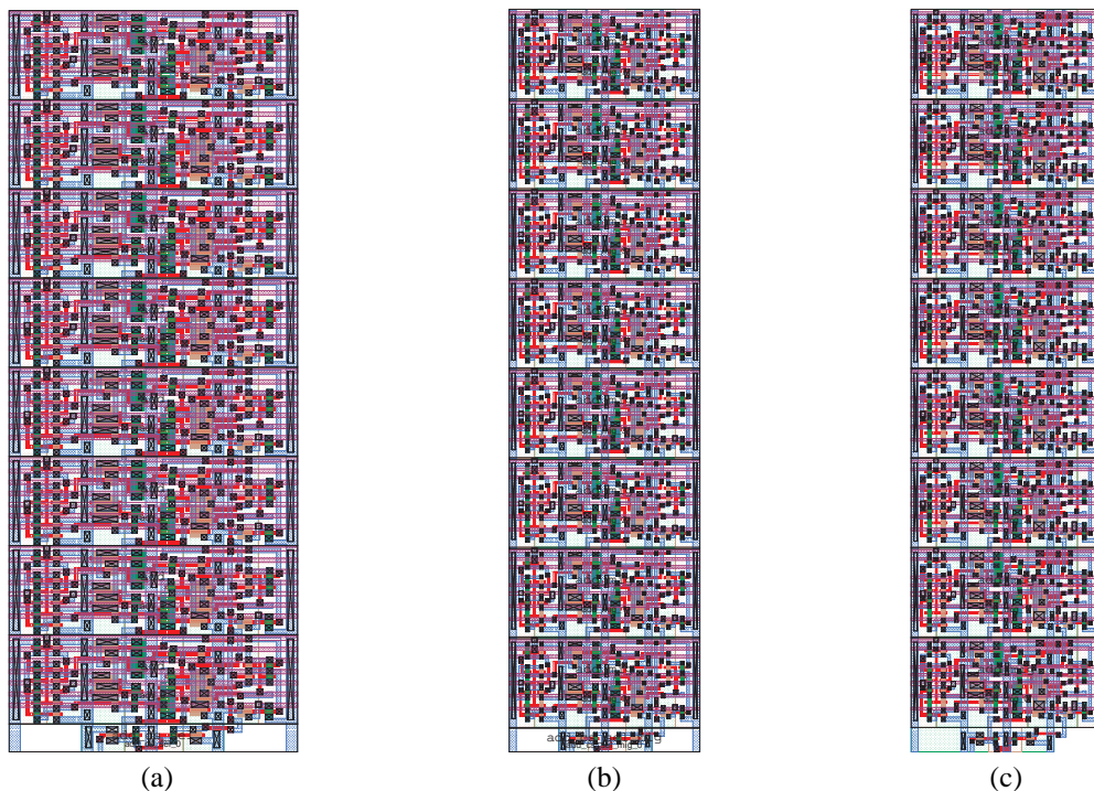
Fig. 6. Migration of 8-bit adder (a)Original layout; (b) Migrated layout in TSMC 0.25 \mu\text{m} ; (c) Migrated layout in TSMC 0.18 \mu\text{m} .
