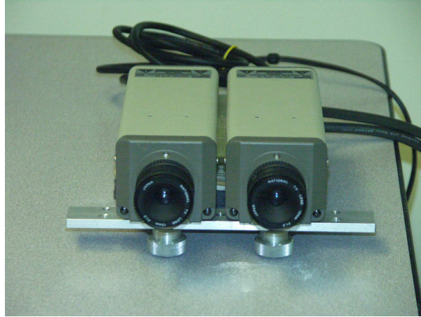
Figure 3.16: The stereo-rig with two NTSC cameras. The separation between the optical centres of the two cameras is approximately 70mm.
