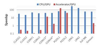
Figure 2: Speedup of GPU over CPU (SIMD) and DianNao accelerator [5].
