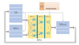
Figure 3: Block diagram of the DianNao accelerator [5].
