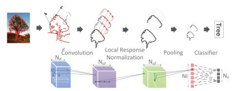
Figure 1: The four layer types found in CNNs and DNNs.
