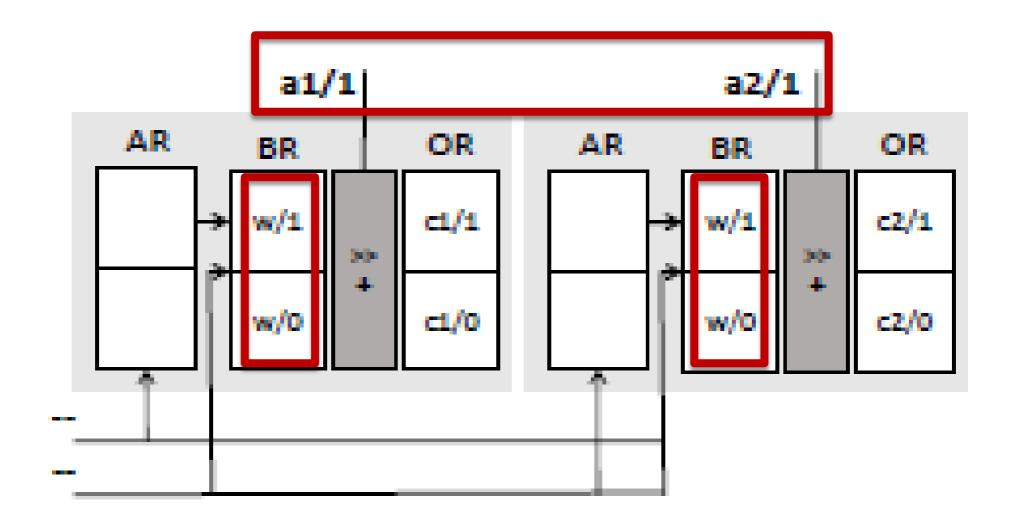
3-stage pipeline to do 2: 2b activation x 2b weight
