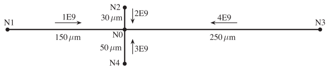
Fig. 20. Layout for a 4-line configuration at a plus-junction.
