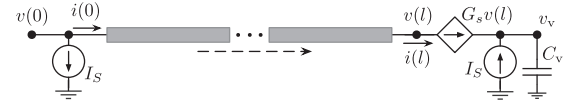
Fig. 13. Equivalent circuit (version 3) for a line with a void at x = l .
