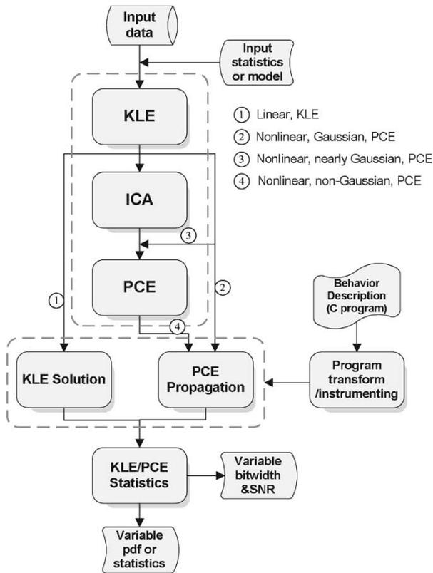
Fig. 5. Block diagram of PCE/KLE method.
