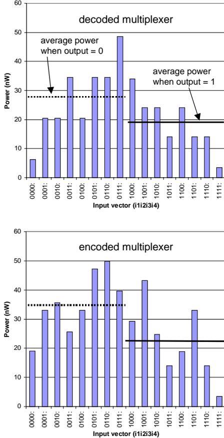
Fig. 4. Leakage power for multiplexers.
