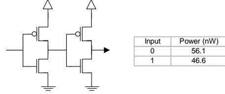
Fig. 6. Buffer implementation and leakage power.
