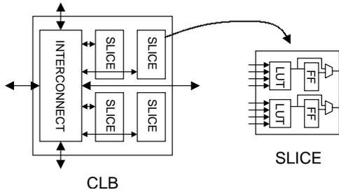
Fig. 11. Configurable logic block (CLB) tile.
