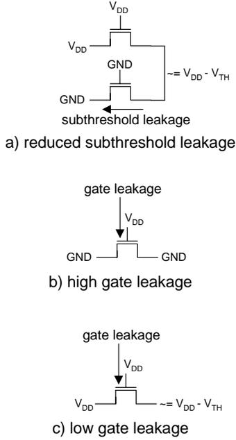
Fig. 5. Examples of transistor leakage states.
