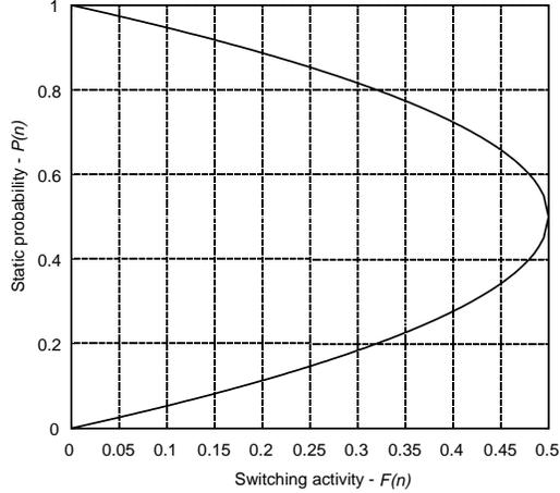
Fig. 10. Static probability versus switching activity.
