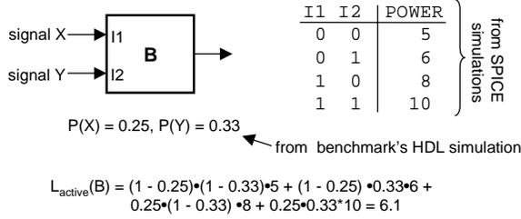
Fig. 13. Example active leakage power computation.
