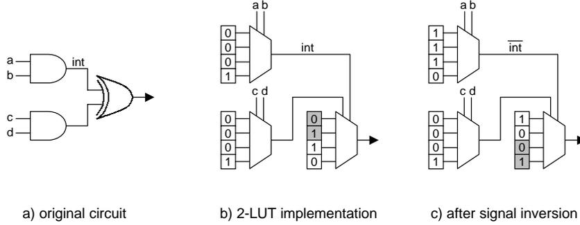
Fig. 8. LUT circuit implementation; illustration of signal inversion.
