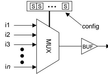
Fig. 2. Routing switch.
