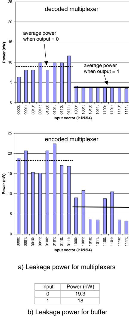
Fig. 7. Low temperature leakage power results for multiplexers and buffer (40°C).
