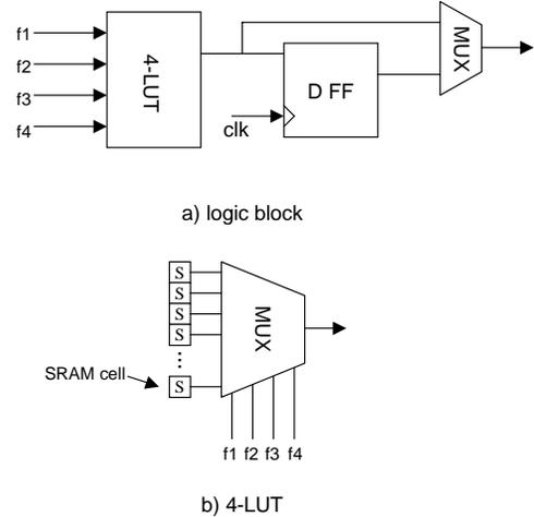
Fig. 1. FPGA logic block.
