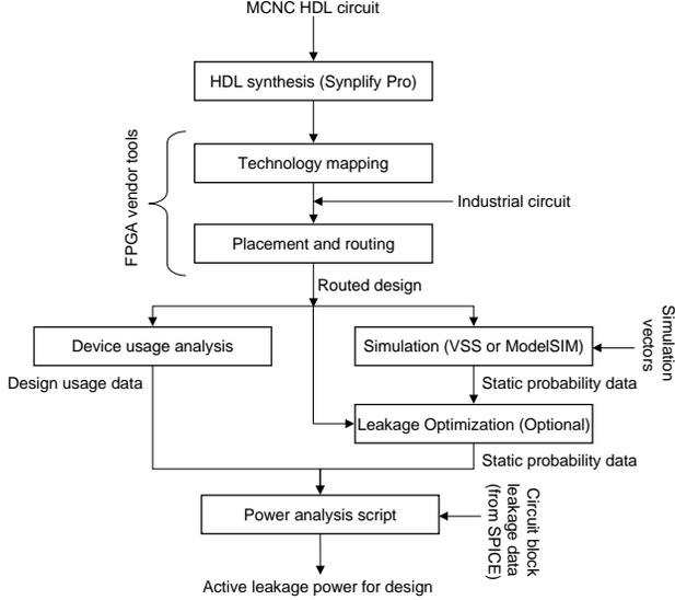
Fig. 12. Leakage analysis flow.
