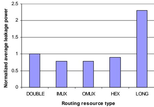
Fig. 16. Average leakage of routing resource types.
