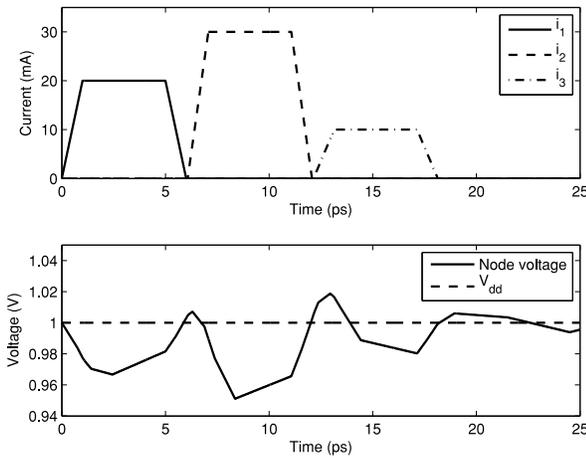
Fig. 2. Current configuration resulting in a large overshoot.
