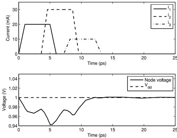
Fig. 3. Current configuration resulting in a small overshoot.
