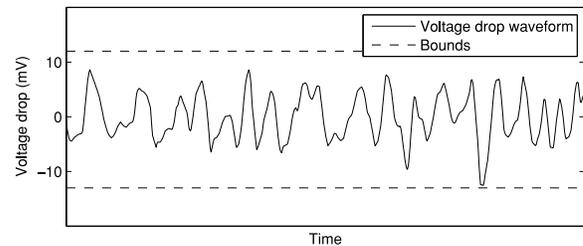
Fig. 6. Voltage drop waveform and bounds at node 4000 in the 4075-nodes grid.
