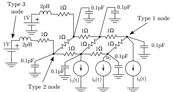
Fig. 1. Small RLC power grid.
