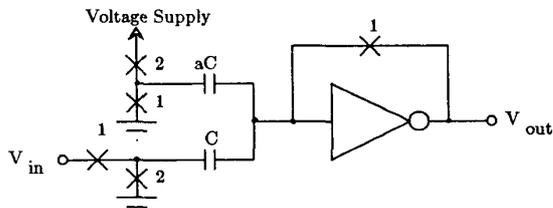
FIG 2 Charge-Subtraction Threshold Detector
