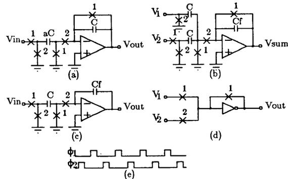
FIG 1 (a) Gain Stage, (b) Adder, (c) Integrator, (d) Comparator, (e) Clock signals
