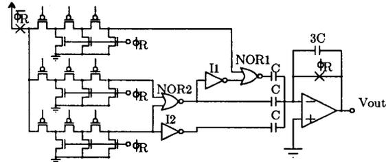
FIG 12 Quaternary SC-Pass-Transistor Circuit \*
