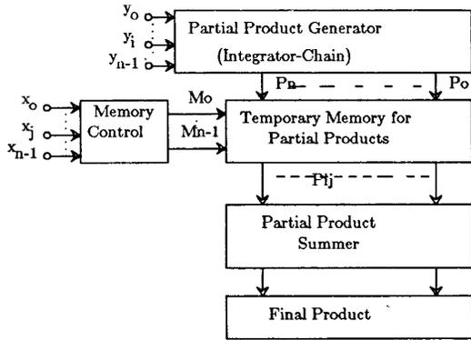
FIG 6 Block Diagram for the SC NxN Multiplier
