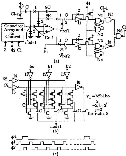
FIG 7 (a) One Stage of the Integrator-Chain
