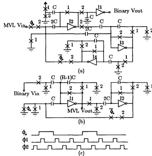
FIG 3 (a) MVL-to-Binary Converter
