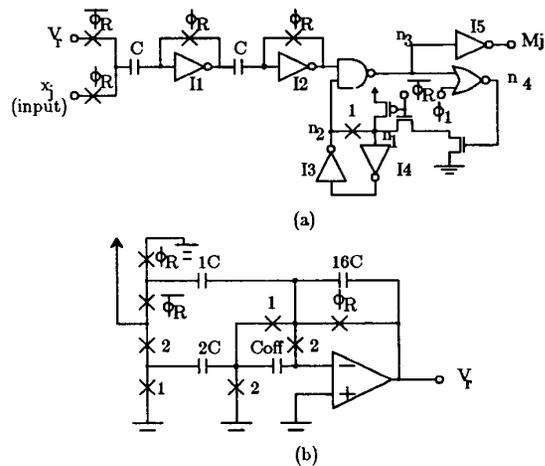
FIG 8 (a) Memory Control Comparator
