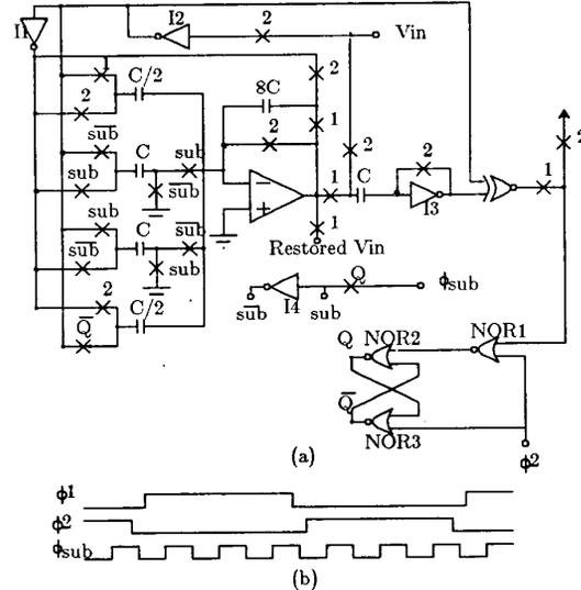
FIG 5 (a) MVL Regenerator for Radix 8
