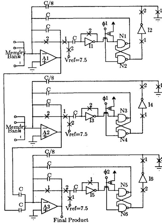
FIG 10 Serial Adder for 4x4 Multiplication
