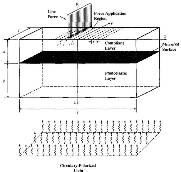
Fig. 1. Two-layer photoelastic transducer.
