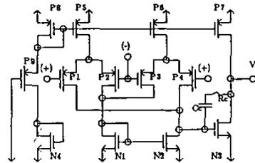
Fig. 3: A three-input amplifier implementation
