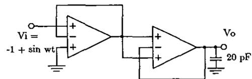
Fig. 4: The setup for measurement of THD
