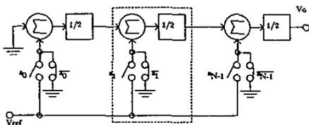
Fig. 1: D/A converter using voltage summers
