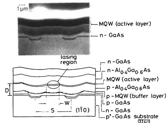
Fig. 1 Scanning electron micrograph of laser cross-section (top) and schematic drawing (bottom) of laser structure
