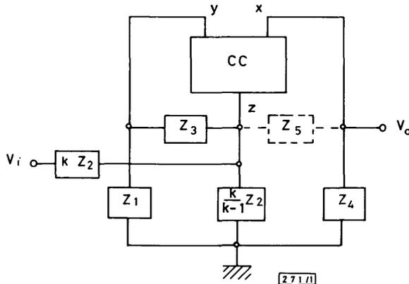
Fig. 1 Four- or five-variable configuration
