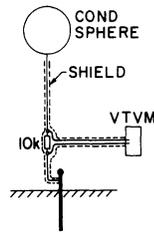
Fig. 2. Arrangement for potential measurement.
