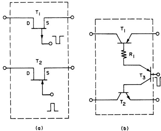
Fig. 5. Simple current switches.
