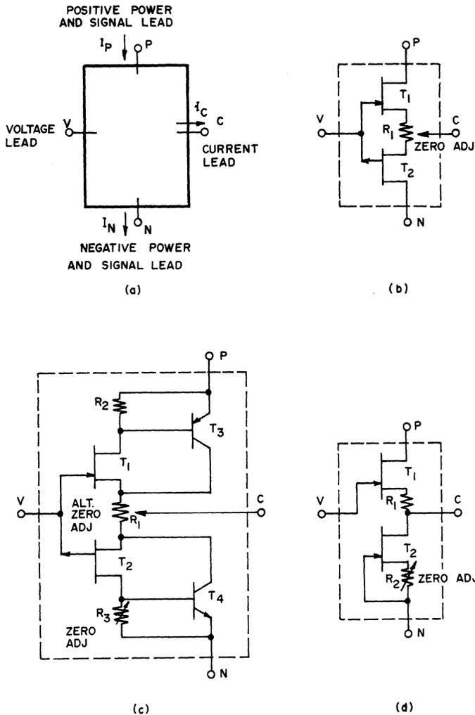
Fig. 2. Typical buffer elements receiving power from and transmitting differential signals on connecting shielded twisted pair. All FET's should be in close thermal proximity.
