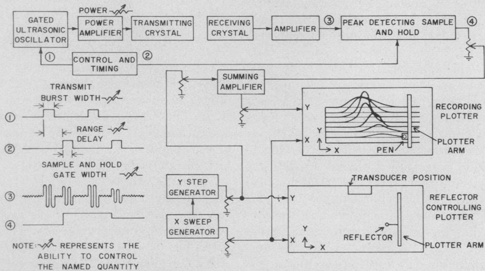
Fig. 3. Field pattern visualization instrumentation.
