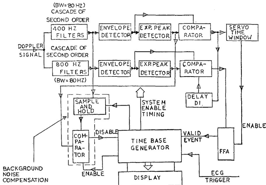
Fig. 2 Block diagram of p.e.p. monitor
