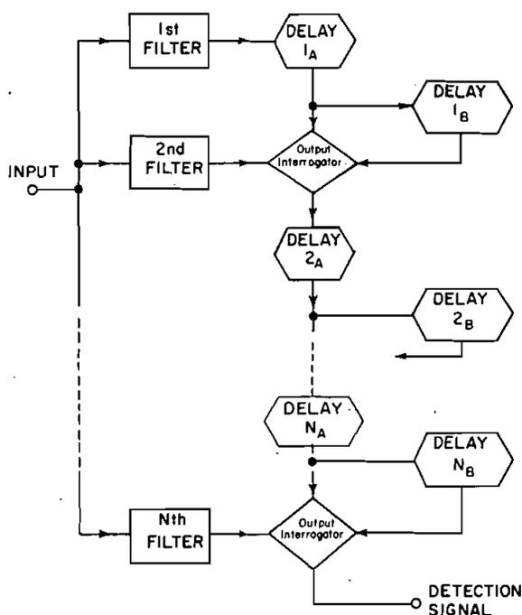
Figure 1. Block diagram of sequential transient filtering technique.
