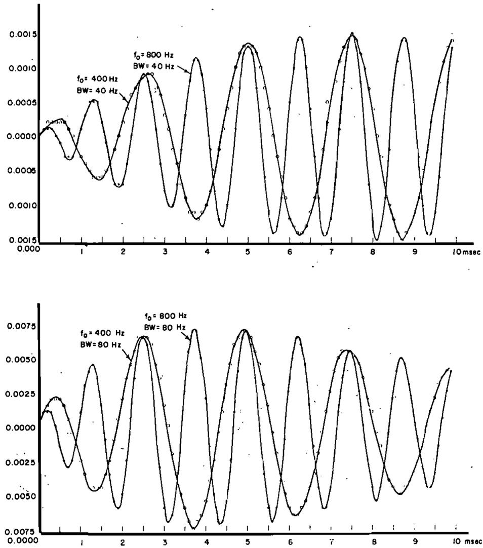
Figure 5. Impulse response of equal  $BW$  bandpass filters.
