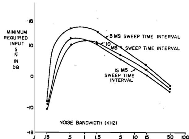
Figure 4. Empirical plot of inherent signal to noise ratio as a function of sweep rate and noise bandwidth.
