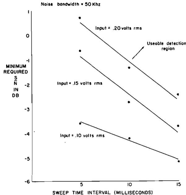
Figure 3. Empirical plot of inherent signal to noise ratio as a function of signal amplitude and sweep-time interval.
