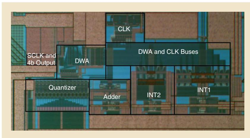
**ISSCC** **FIGURE 16:** A power-efficient direct-charge-transfer adder with timing modification.
