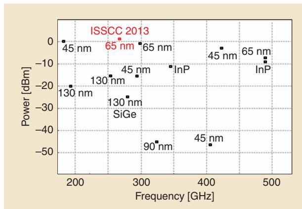
**FIGURE 18:** Output power versus frequency for mm-wave and sub-mm-wave sources.
