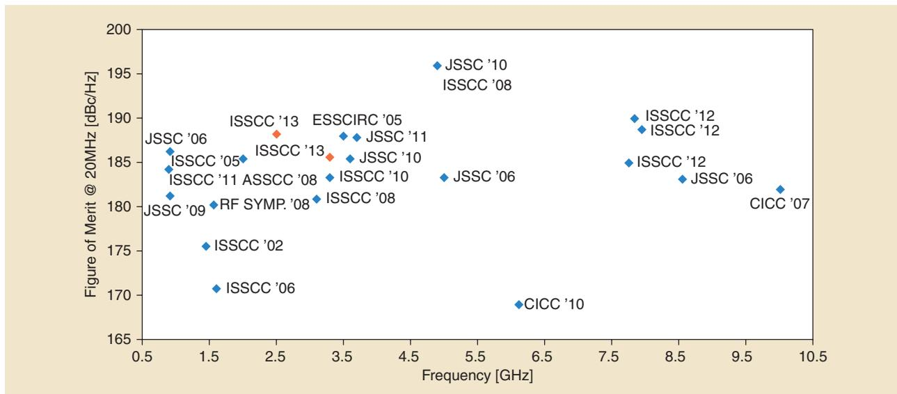
**FIGURE 19:** Phase-noise FoM at 20-MHz offset frequency versus oscillation frequency.
