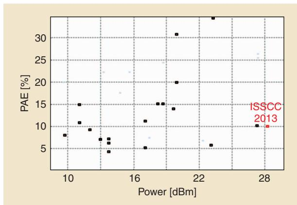
**FIGURE 17:** PAE versus output power for recent submicron mm-wave CMOS PAs.
