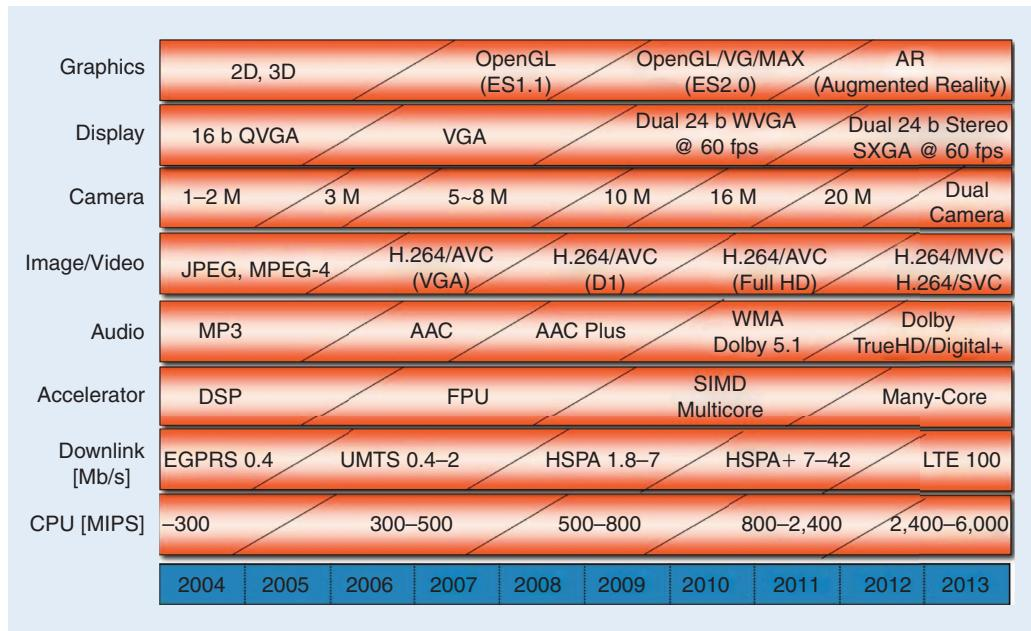
**FIGURE 5:** Developments in application processors for smartphones.
