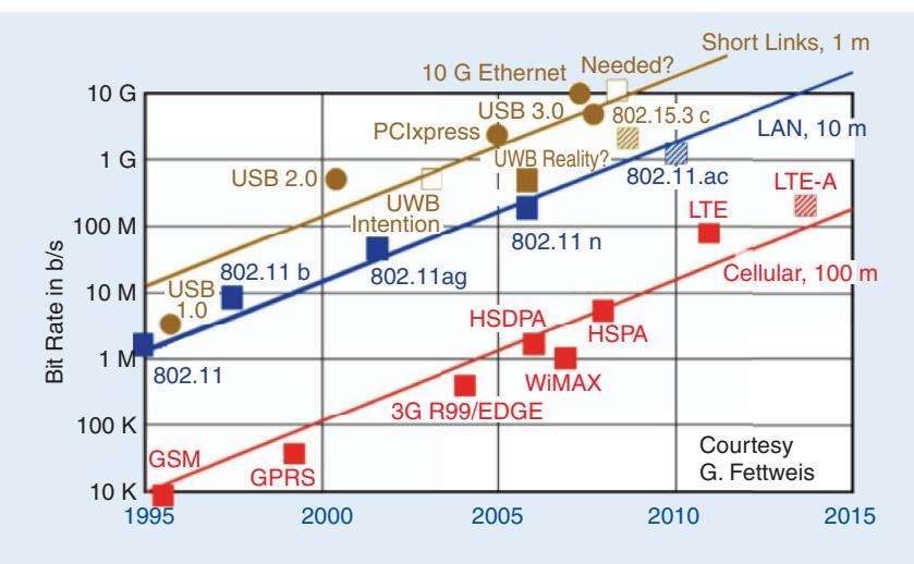
**FIGURE 6:** Wireless and wired data rates over time. (Image courtesy of G. Fettweis.)
