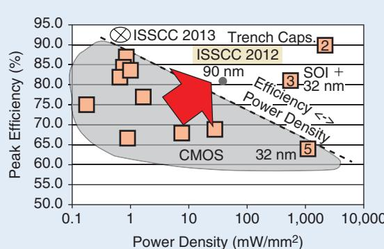
**FIGURE 1:** The development of integrated power conversion: Each year, more and more are integrated in standard CMOS technologies, optimizing efficiency versus power density. At ISSCC 2013, these trends are evident in a shift to higher performance, as shown by the arrow directed to the upper right. (Adapted, courtesy of ISSCC 2012 Paper 5.4.)
