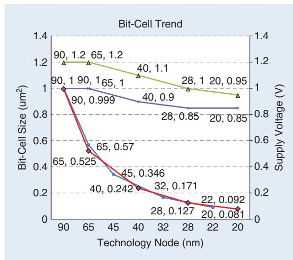
**FIGURE 12:** SRAM bit-cell size and supply scaling range from major semiconductor manufacturers.
