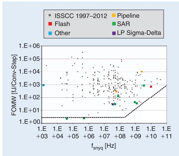
**FIGURE 3:** FoM (energy per conversion step) versus Nyquist bandwidth for various converters.
