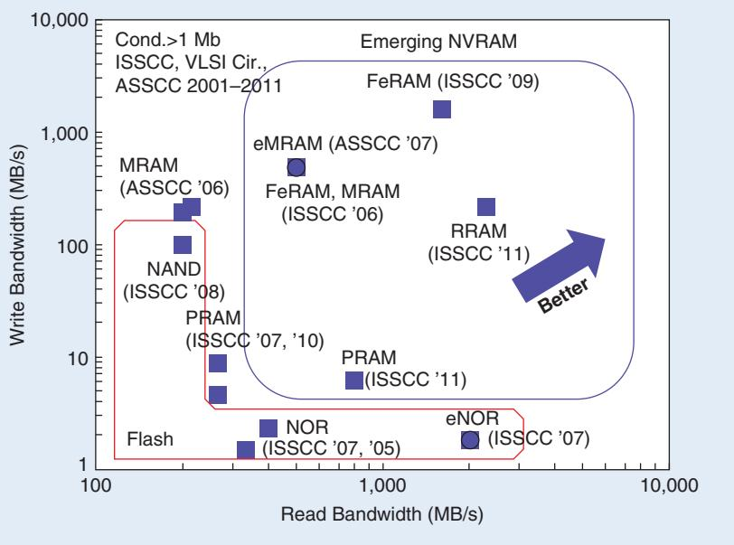
**FIGURE 14:** Read- and write-bandwidth comparison of nonvolatile memories.
