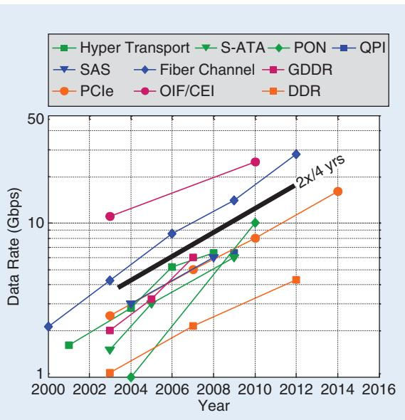
**FIGURE 22:** Per-pin data rate versus year for a variety of common wireline I/O standards.
