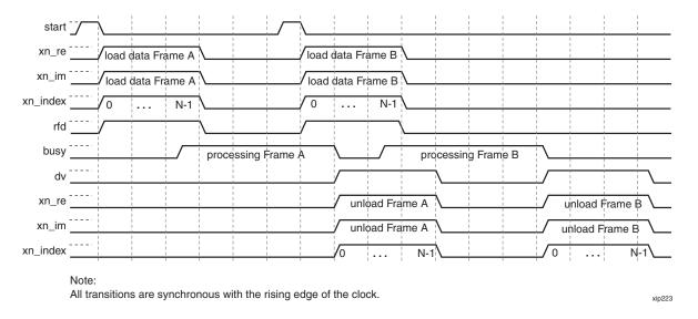
Figure 9: Timing for Non-Continuous Data Stream
