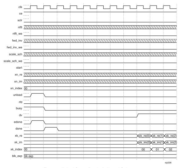
Figure 11: Unload Output Results in Natural Order
