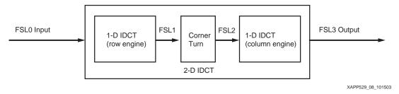
Figure 8: Block Diagram for using a 1-D IDCT to implement a 2-D IDCT
