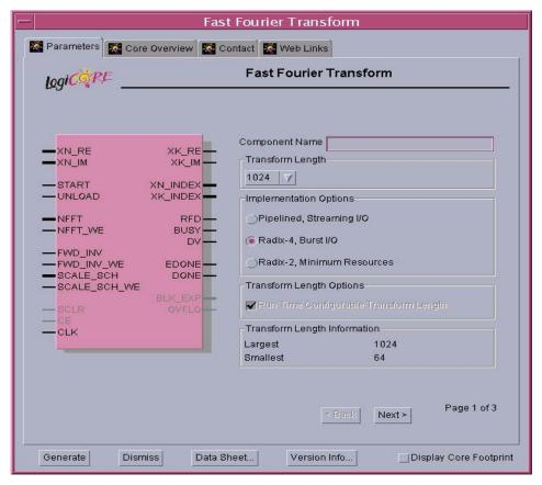
Figure 5: XFFT Core GUI Main Window
