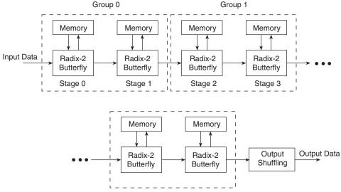
Figure 1: Pipelined, Streaming I/O
