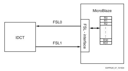
Figure 7: Including the 1-dimensional IDCT IP via the FSL interface onto MicroBlaze
