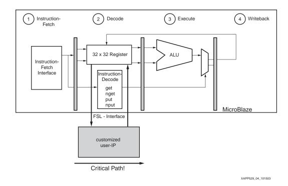
Figure 4: Including a customized IP via the FSLinterface onto MicroBlaze
