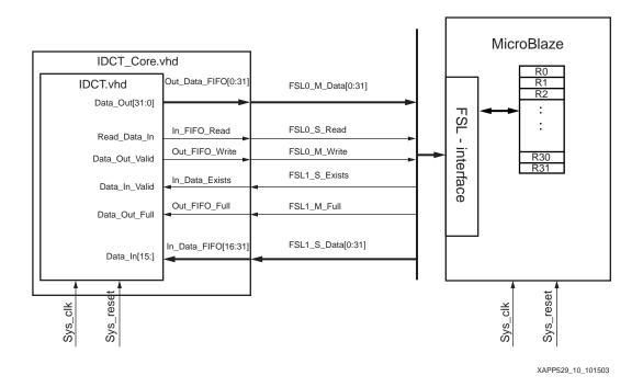
Figure 10: Figure 10: Detailed connection of the 1-dimensional IDCT IP to MicroBlaze
