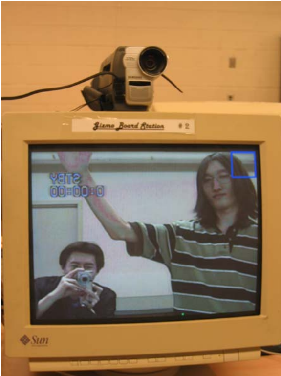
Figure 5 – Note how the video input is horizontally flipped when we show the camera's status. This was necessary so that the user's left hand would appear on the left side of the monitor: otherwise gameplay would be very confusing!
