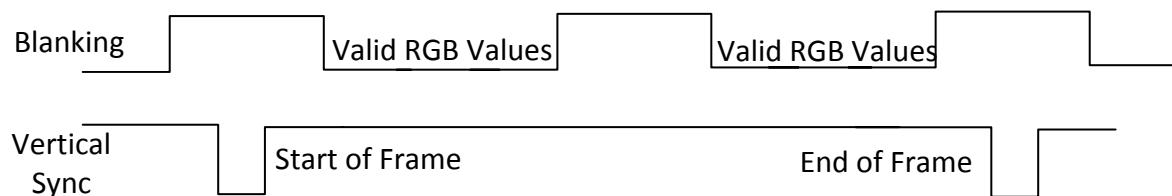
Figure 6 - VGA Timing Signals
