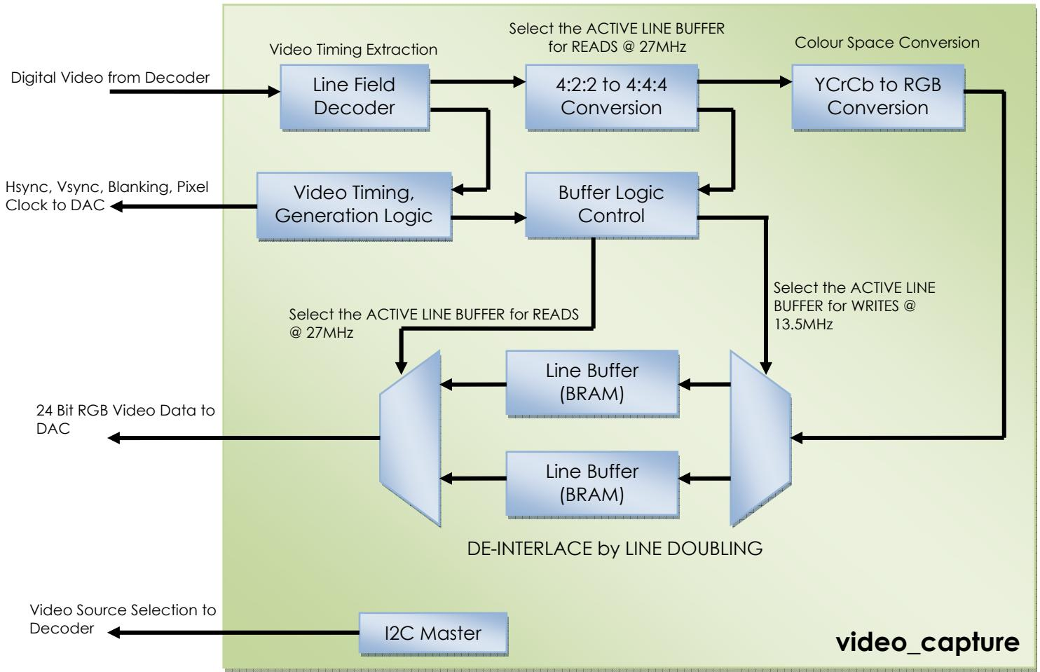
Figure 4 - Video Capture Block Diagram
