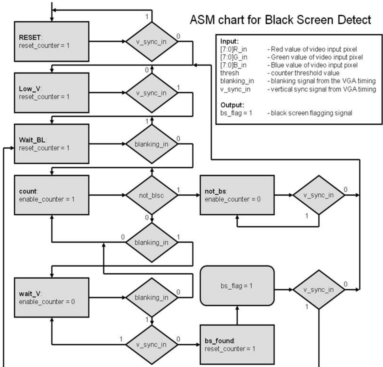
Figure 7 - Black Screen Detect ASM Chart
