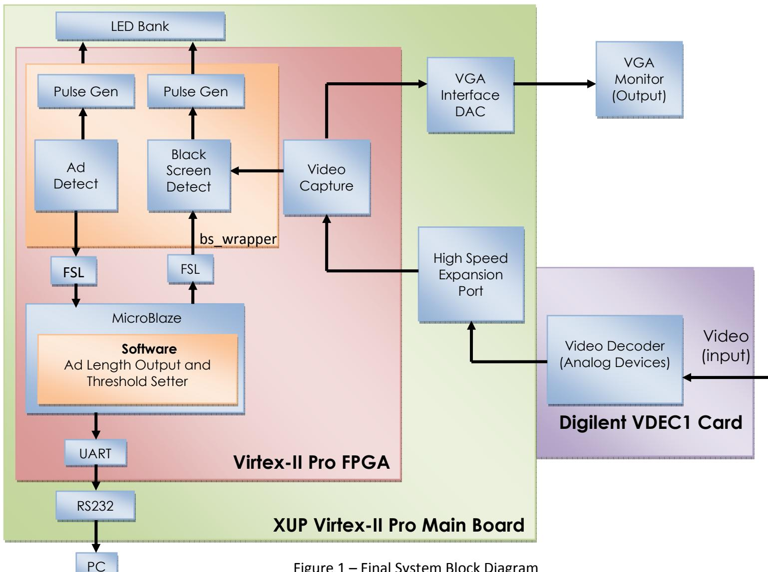
Figure 1 – Final System Block Diagram
