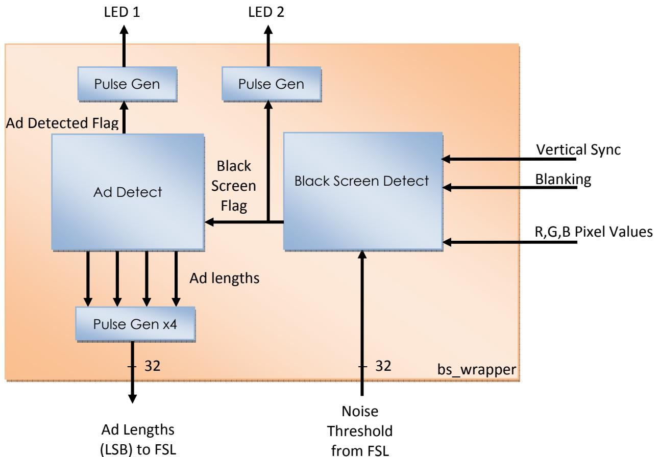
Figure 5 - bs\_wrapper Block Diagram
