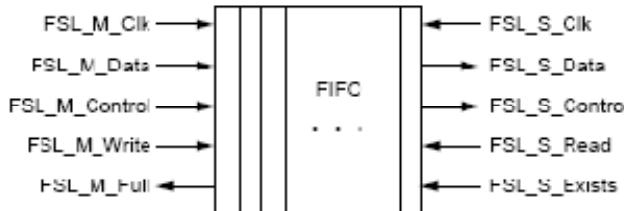
Figure 3 - Fast Simplex Link (FSL) Block Diagram
