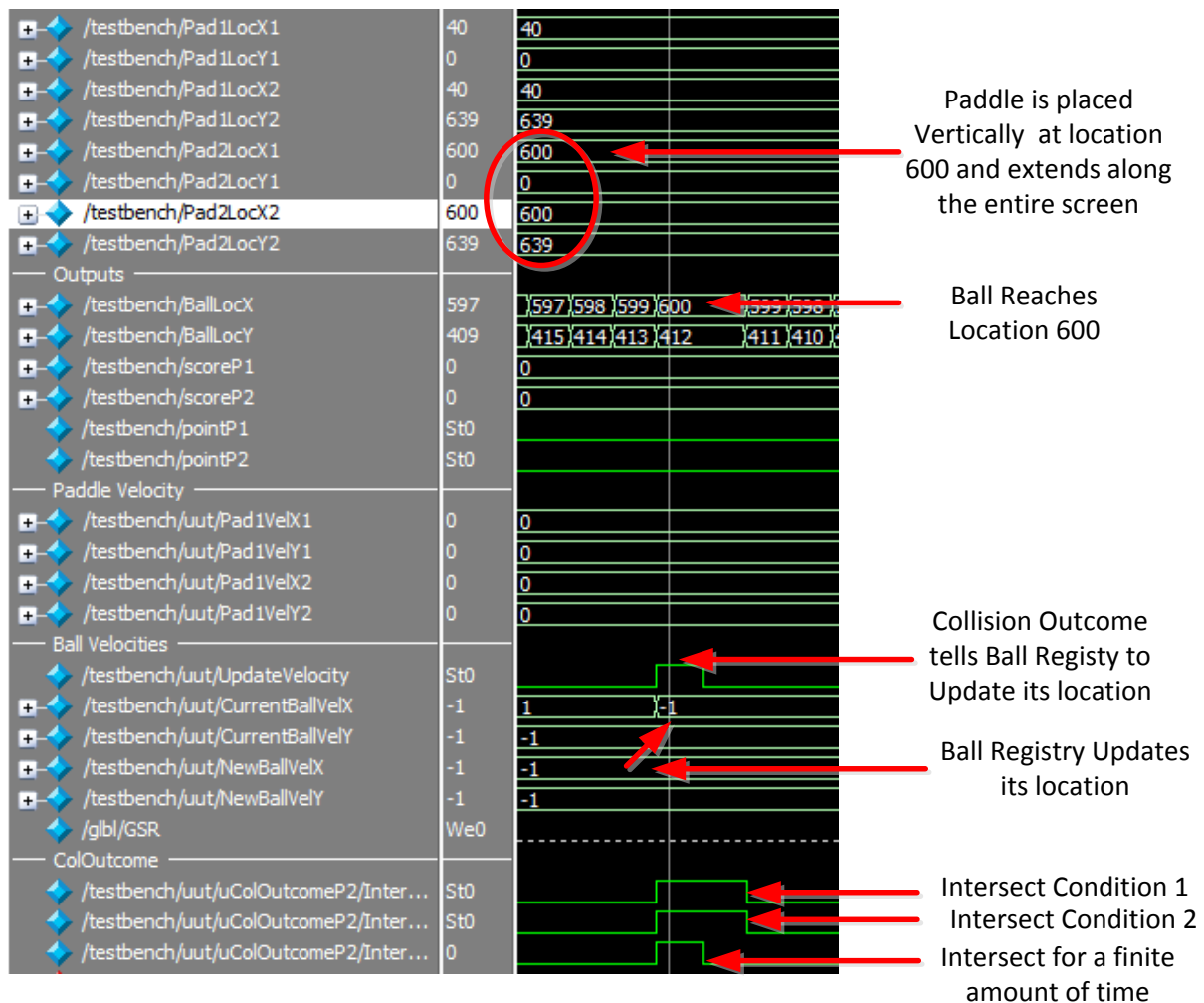
Figure 21 ModelSim simulation. Basic case depicting a collision of a stationary paddle with a moving ball
