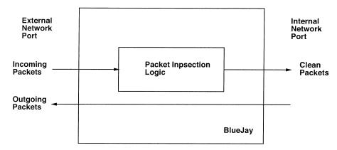
BlueJay will have two ethernet connections: an *External* port for connecting to the outside world and an *Internal* port for the internal network. The ethernet should be capable of running up to the 1 GigE standard (Gigabit Ethernet). Incoming packets are buffered in memory by one process. A separate process removes the packets from memory and runs them through the packet inspection logic.
