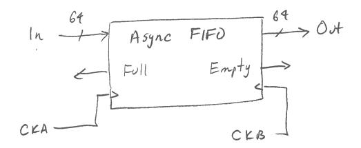
The async FIFO is built with an async memory (no clock) that has 2 ports. Read and write Can be done at different speeds
