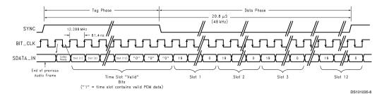
FIGURE 6. AC Link Audio Input Frame
