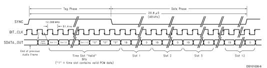
FIGURE 4. AC Link Audio Output Frame
