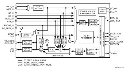
FIGURE 1. LM4549 Block Diagram
