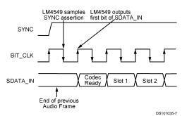
FIGURE 7. Start of Audio Input Frame
