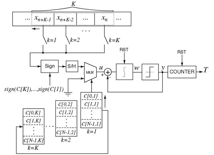
Fig. 5.  $\Delta\Sigma$ -modulated FIR filter.
