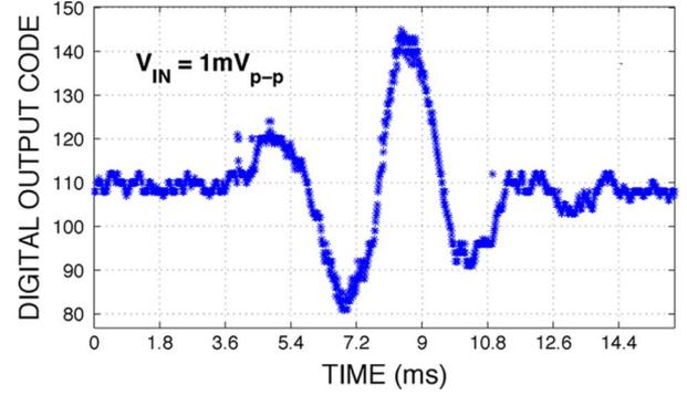
Fig. 13. Measured digitized output of the full recording channel including the amplifier and ADC with an emulated neural spike input of  $1 \text{ mV}_{pp}$ .
