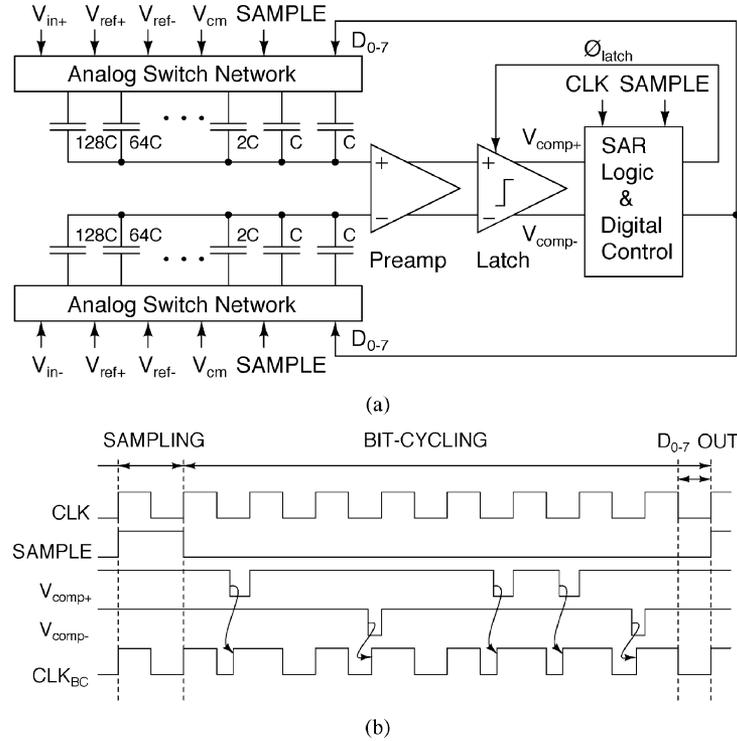
Fig. 10. (a) Self-timing successive approximation ADC architecture. (b) Sample timing diagram of the SAR ADC.
