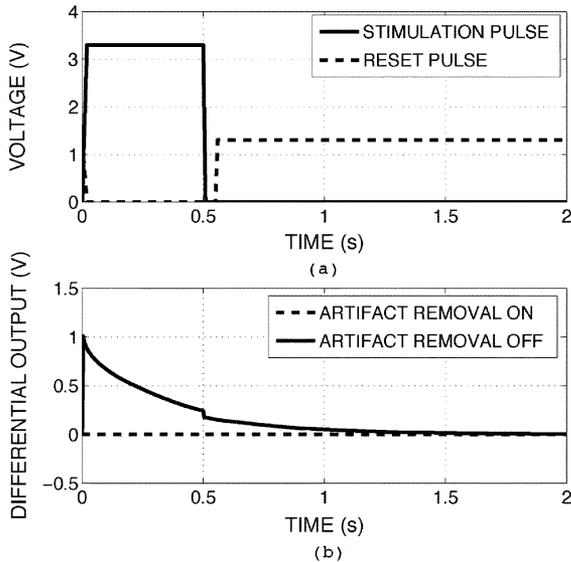
Fig. 17. (a) Stimulation pulse applied to the input of the recording amplifier with a corresponding reset signal to minimize artifacts. (b) Output of the recording amplifier with and without a reset signal applied to the feedback transistor.
