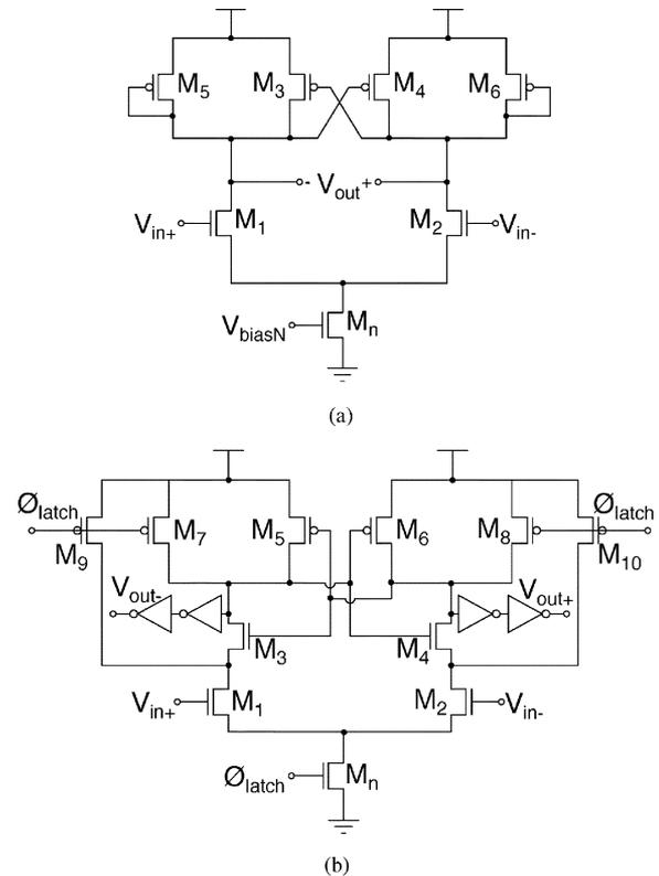
Fig. 11. (a) Preamplifier and (b) comparator circuits.
