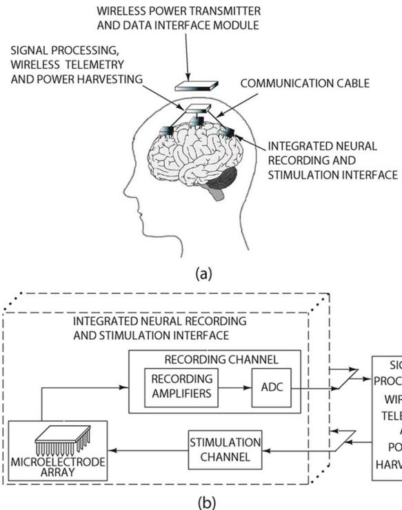
Fig. 1. (a) Implantable system for cortical recording and stimulation. (b) Block diagram of the implanted components of the system.
