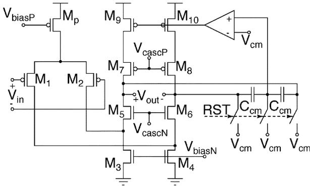
Fig. 9. Fully differential folded cascode OTA.
