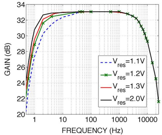
Fig. 8. Measured amplitude frequency response of the first-stage amplifier with programmable HPF cutoff frequency adjusted by changing the bias voltage of feedback resistors  $V_{res}$ .
