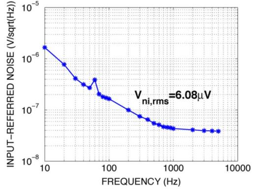
Fig. 7. Measured input-referred voltage noise density for the first stage of the amplifier between 10 Hz and 5 kHz.
