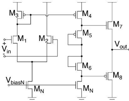
Fig. 16. Class AB buffer output stage.
