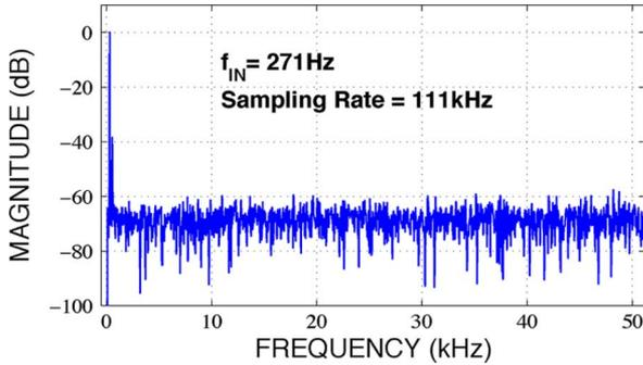
Fig. 12. Measured output spectrum of ADC for a 271-Hz sinusoid input sampled at 111 kilosamples/s.
