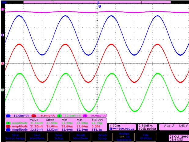
Fig. 6. Output of three different neural channels, with a 0.8-mV input (top waveform).
