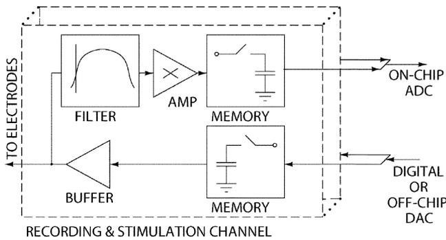
Fig. 3. Architecture of one column of the neural recording and stimulation interface. Each recording amplifier and stimulator is in-channel and the ADC is column parallel.
