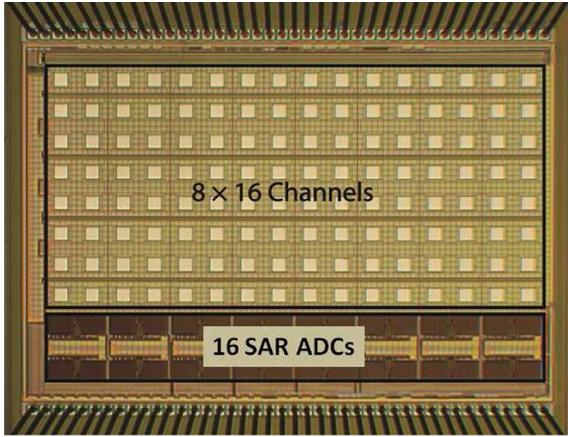
Fig. 2. Micrograph of the neural recording and stimulation interface.
