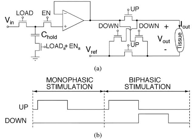
Fig. 14. (a) In-channel voltage-mode biphasic stimulator. (b) Stimulator timing diagram.
