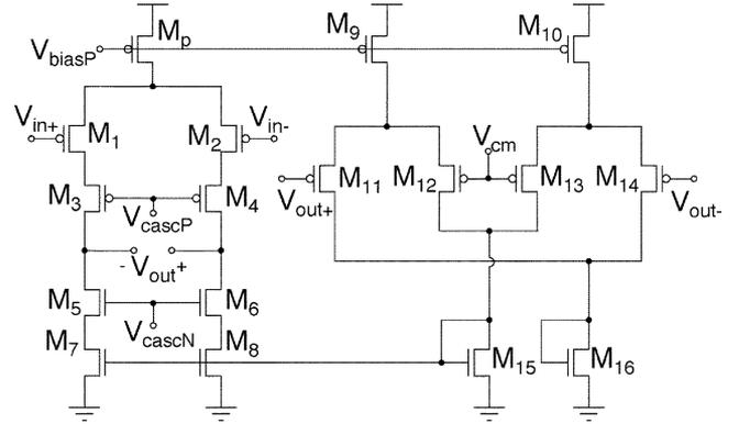
Fig. 5. Fully differential telescopic OTA.
