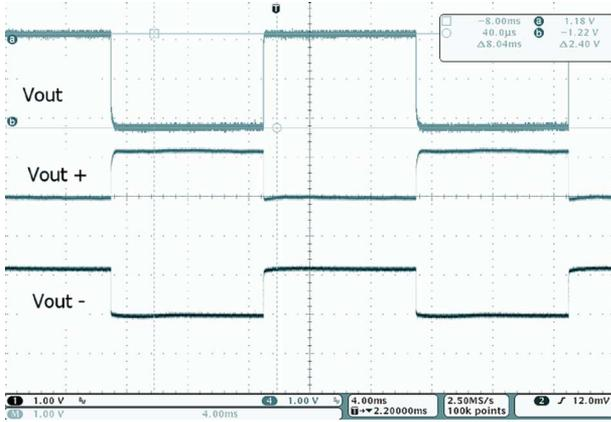
Fig. 15. Experimentally measured biphasic voltage stimulator output.
