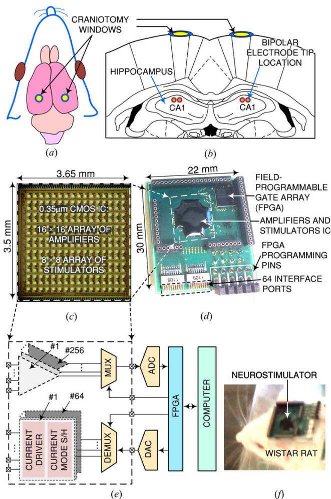
Fig. 3. Bipolar electrode implantation: (a)–(b) locations of craniotomy windows and implanted electrode tips; (c) bi-directional neural interface custom integrated circuit with 256 neural amplifiers and 64 neurostimulators; (d) custom-made programmable therapeutic neurostimulation device with 64 recording channels or 64 stimulation channels enabled; (e) system-level block diagram; and (f) a freely moving rat with the neurostimulator mounted on the head to demonstrate the form factor.
