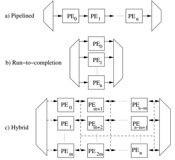
Figure 2: Parallelization models.
