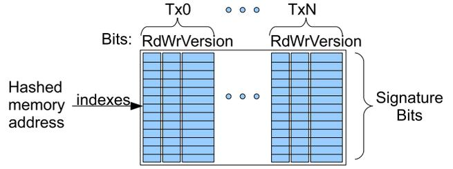
**Figure 6: Signature table used to mark speculatively read and/or written for N hardware contexts. Version bits are used to distinguish between consecutive transactions on the same hardware context: a mismatch between this version and the context’s transaction number indicates that the entry for that context is invalid.**
