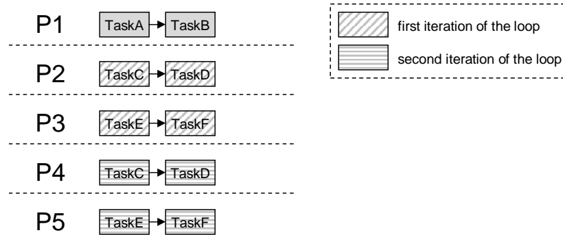
Figure 5.7: The run-time execution of tasks after buffer privatization for the running example.
